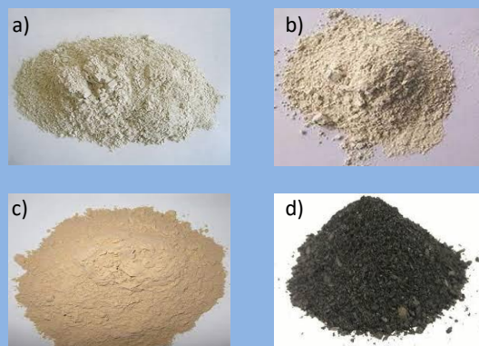
Fig. 1. Adsorbents matrices: a) zeolite, b) attapulgite, c) bentonite, d) biochar
